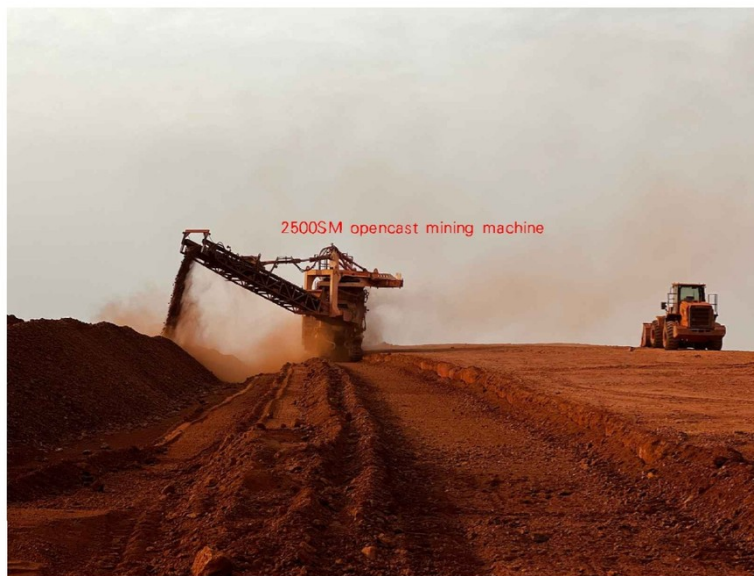
Fig. 13-1 Operation of the 2500SM Opencast Mining Machine
